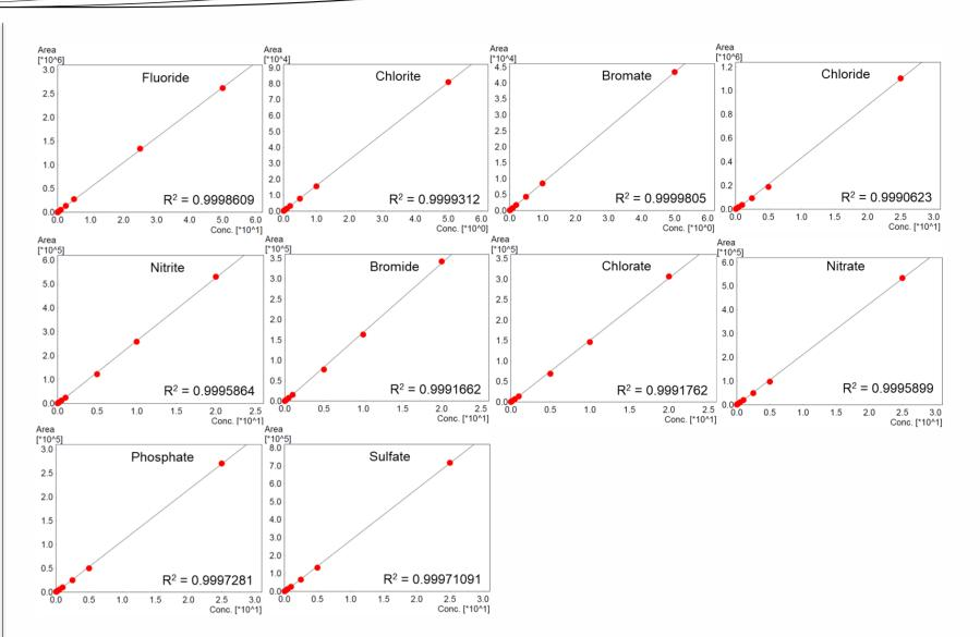
Fig. 4 Calibration curves for 10 anions listed in EPA Method 300.1
