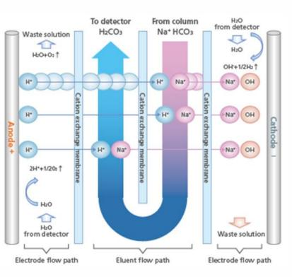
Cations in mobile phase are exchanged with hydronium ions that are continuously generated from water electrolysis.
